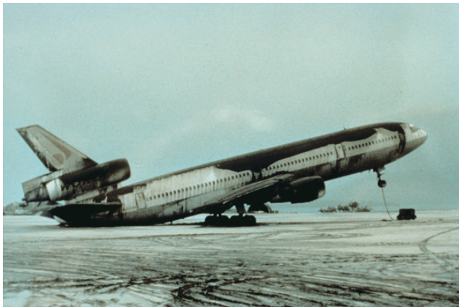
World Airways DC-10, Naval Air Station Cubi Point, on the flight line weighed down by thick, water-soaked ash, June 17, 1991. Photo from U.S. Navy Source: https://seabeemagazine.navylive.dodlive.mil/2018/06/15/kicking-ash-the-seabees-of-operation-fiery-vigil/
