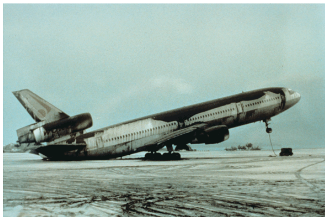
World Airways DC-10, Naval Air Station Cubi Point, on the flight line weighed down by thick, water-soaked ash, June 17, 1991.
