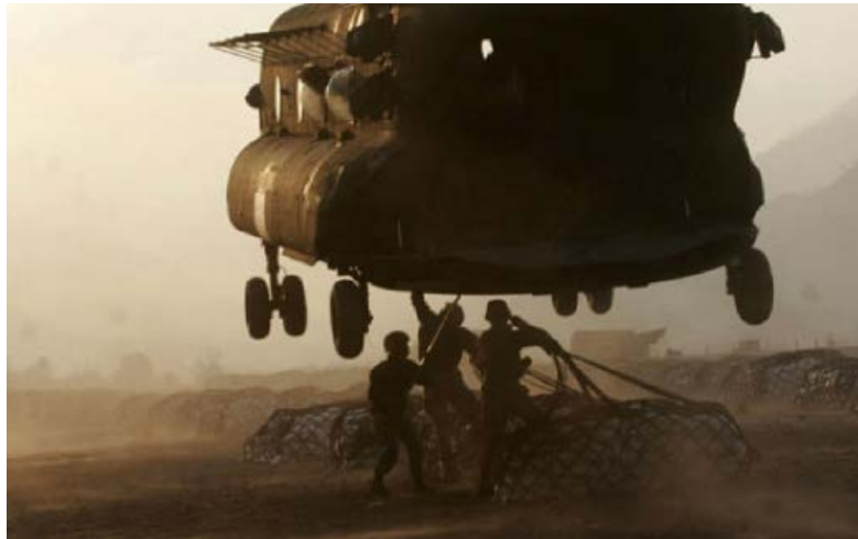
Marine landing support specialists attach external loads, or sling-loads, to the bottom of an Army CH-47 Chinook helicopter in Muzaffarabad, Pakistan. The Okinawa-based Marines served in Pakistan with Combined Medical Relief Team-3. Photo by Scott Biscuiti/USMC Source: https://www.stripes.com/news/okinawa-marines-work-to-get-drop-on-pakistan-quake-relief-1.44356#gallery
