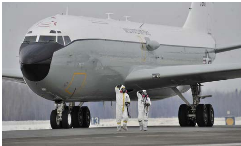
EIELSON AIR FORCE BASE, Alaska -- Personnel from the 55th Aerospace Medicine Squadron and 55th Aircraft Maintenance Squadron report a "thumbs down," which indicates the WC-135 Constant Phoenix aircraft is above acceptable levels of contamination and needs be parked in an isolated location to be decontaminated. This initial radiation survey was done every time the WC-135 landed after collecting air samples in international airspace over the Pacific as part of Operation Tomodachi. Air Force photo by Staff Sgt. Christopher Boitz Source: https://www.afhistory.af.mil/FAQs/Fact-Sheets/Article/690225/operation-tomodachi/
